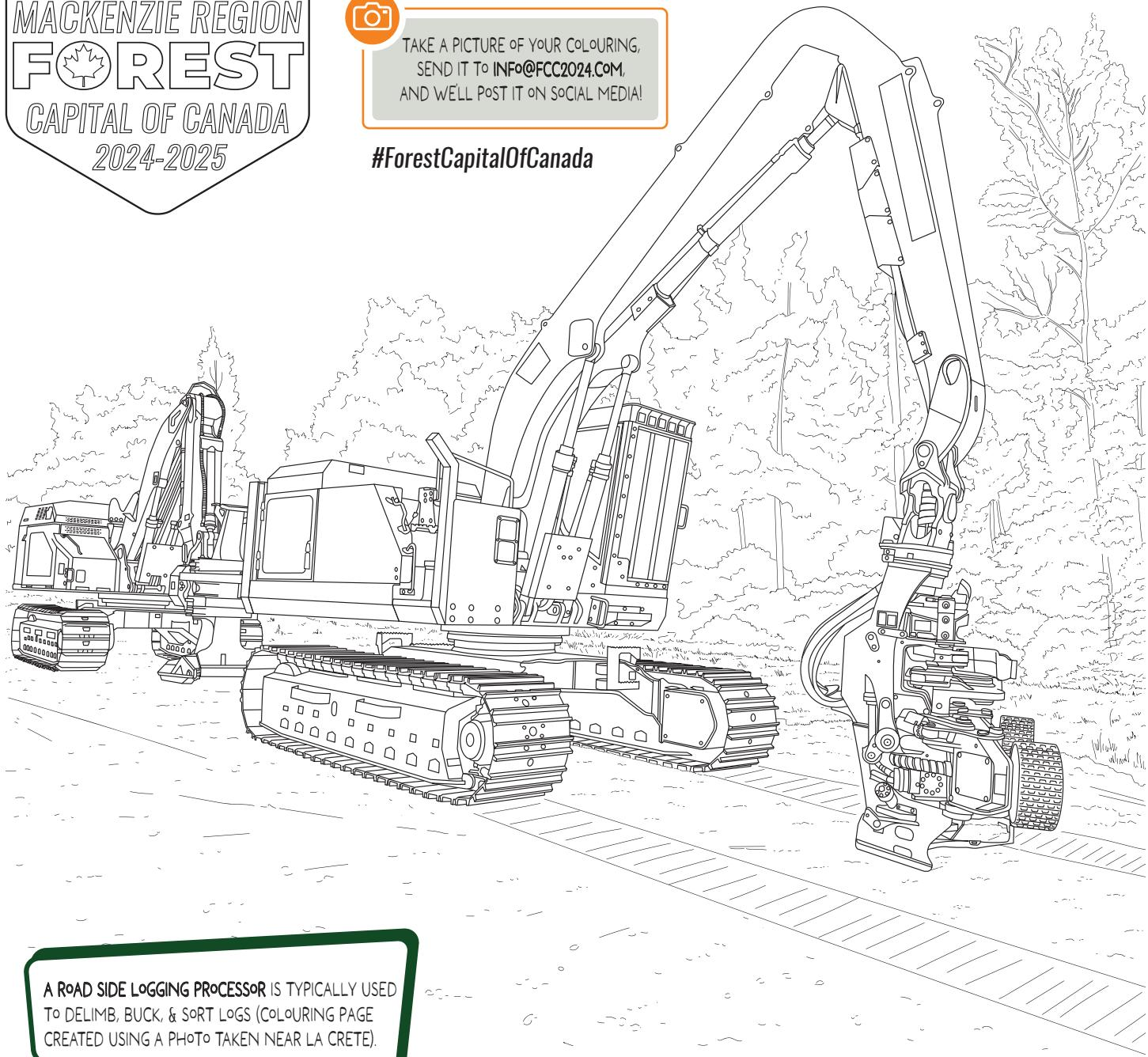
A ROAD SIDE LOGGING PROCESSOR IS TYPICALLY USED TO DELIMB, BUCK, & SORT LOGS (COLOURING PAGE CREATED USING A PHOTO TAKEN NEAR LA CRETE).
